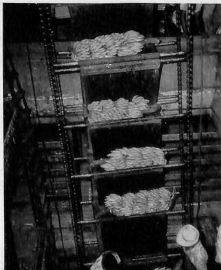
8. DOWN into the hold of ship go the stems of bananas, each one nestling in a pocket of the endless-belt conveyor to prevent rough joggling. Quality of fruit depends on proper handling.
